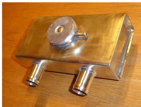
New Header Tank
